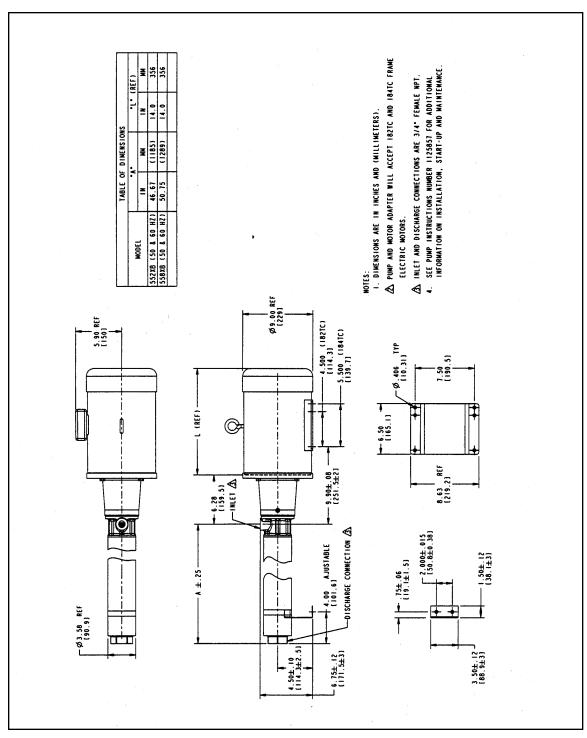
Figure 8.9 500 XB Motor Adapter Pump
